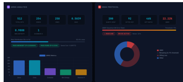
Fig 4: QBER with eavesdropper (web dashboard)
